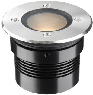
/NGS For maximum lumen output. Deep recessed optic and matt black anodised optic holder aids in glare reduction.
