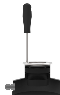
3 Ring is pulled up and expands the O ring, locking fitting into the housing
